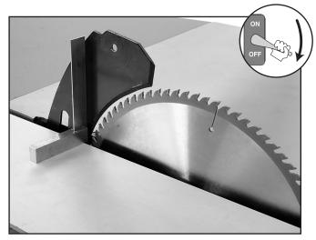
Figure 38. Checking vertical alignment.
